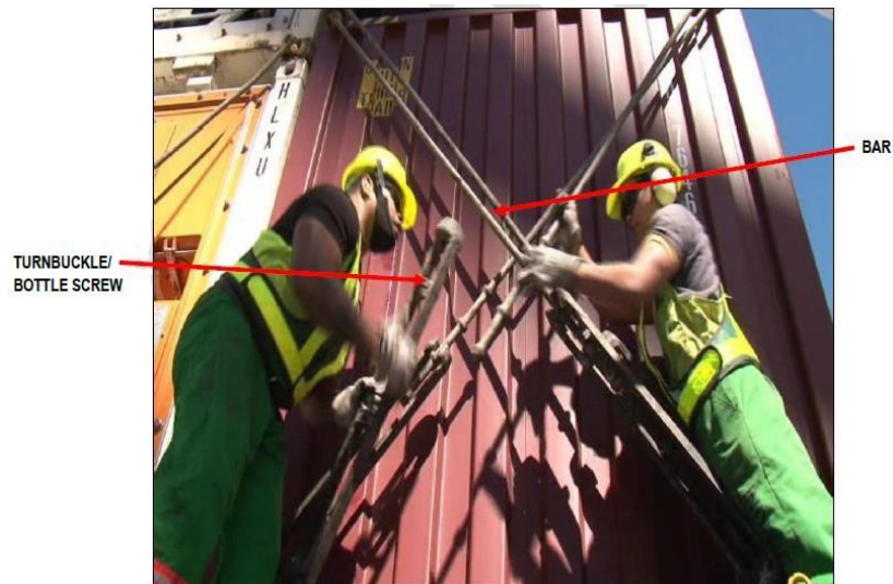
Figure 2: lashers working in pairs showing the components of the lash
